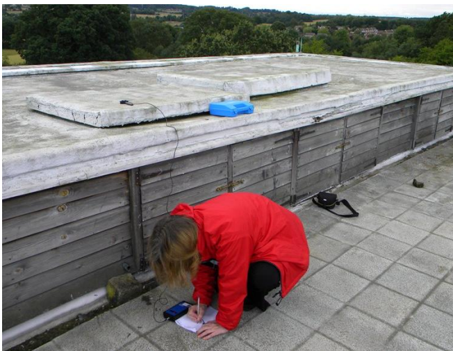
Figure 5 Simultaneous measurement of external horizontal illuminance using a separate light meter.
